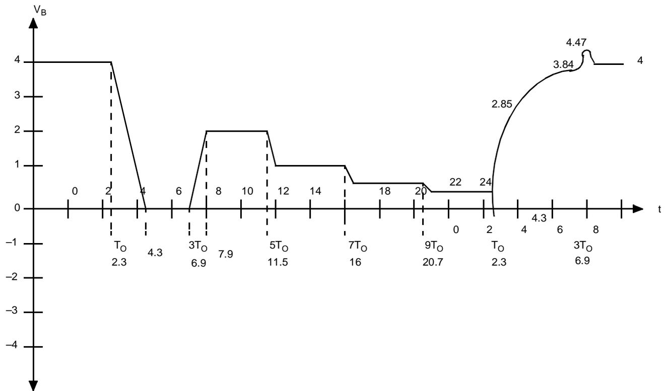
Figure 22b. Underterminated Line Example;  $V_B(t)$
