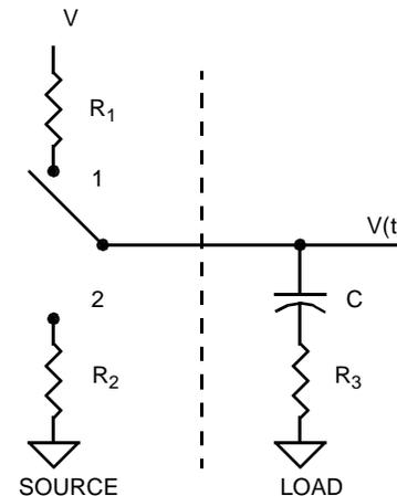
**Figure 18. Lumped Load; AC Termination**
