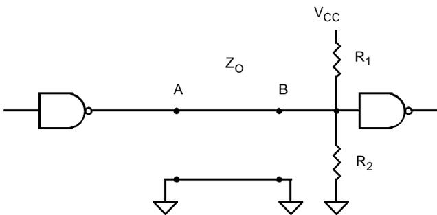
**Figure 16. Pull-Up/Pull-Down**
