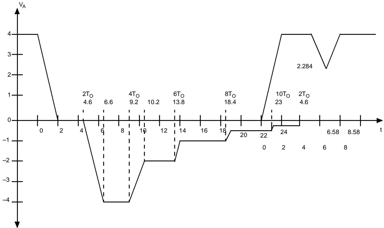
Figure 22a. Underterminated Line Example;  $V_A(t)$
