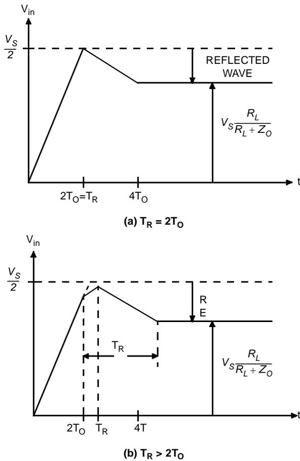
**Figure 9. Effects of Rise Time on Response for  $R_L < Z_O$**
