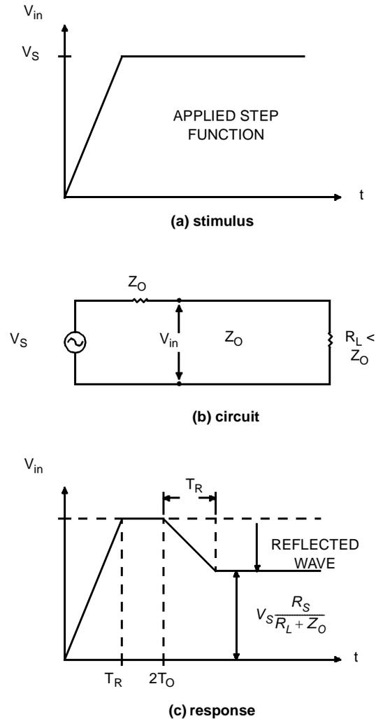
**Figure 8. Effect of Rise Time on Response of Mismatched Line with  $R_L < Z_O$**
