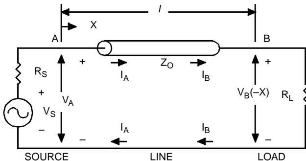
Figure 3. Ideal Transmission Line Loaded and Driven
