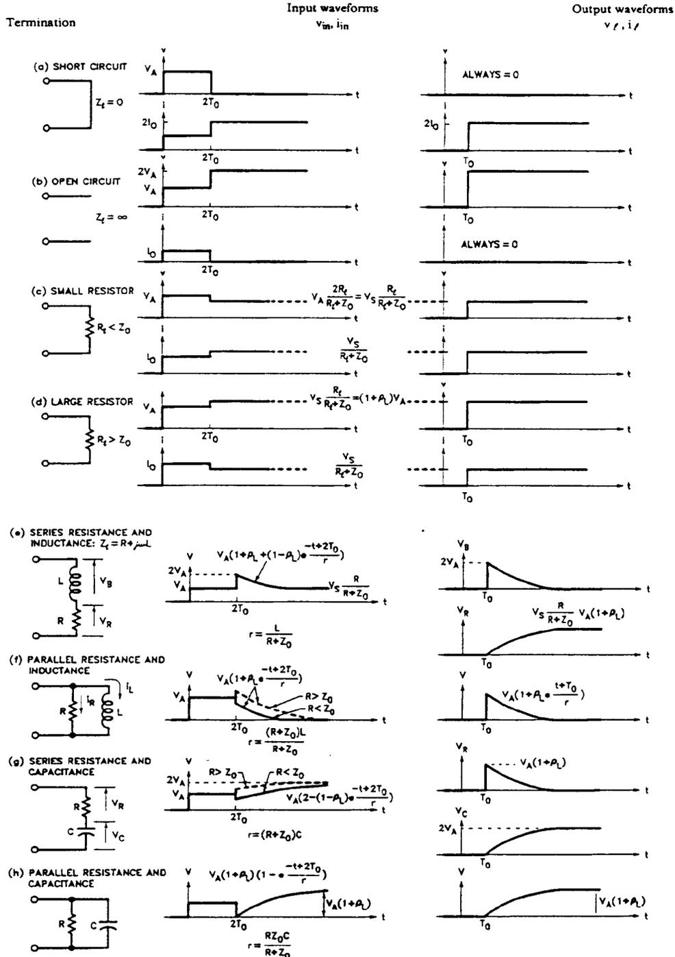
Figure 4. Step Function Response of Figure 3 for Various Terminations
