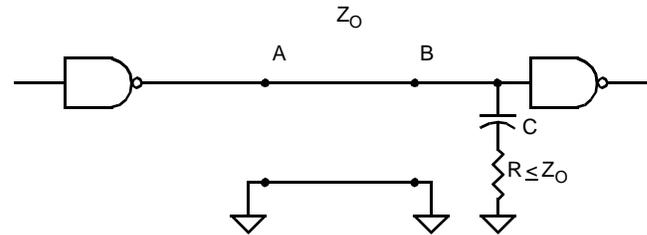
**Figure 17. Parallel AC Termination**
