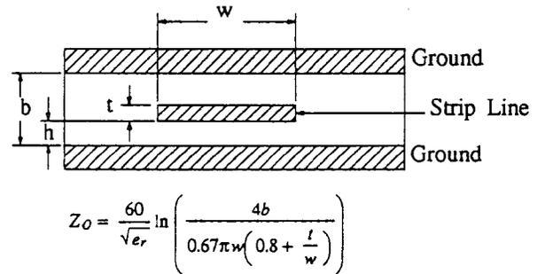
**Figure 13. Strip Line Construction**
